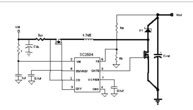
Note: Heavy lines indicate the critical loop carrying high pulsating current. The inductance of the loop needs to be minimized.
