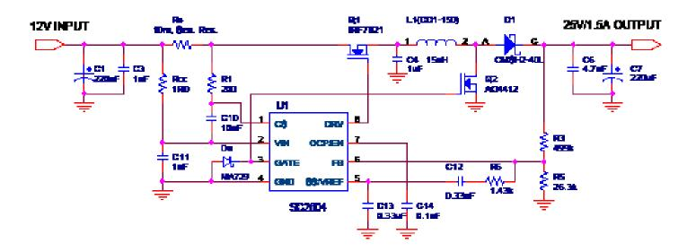
Note: A small Schottky diode (Da) may be required in some applications to clamp negative spike at the GATE pin.
