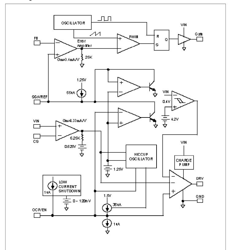
Figure 2. SC2604 Function Diagram
