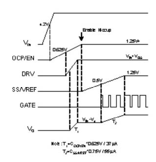
Figure 3. Start-up Timing Diagram
